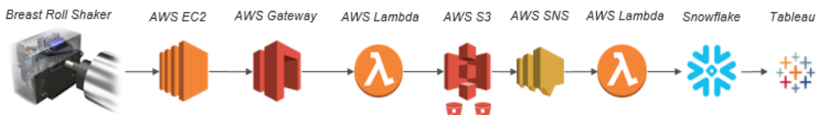
Figure 11. A simplified version of the MCS data pipeline integrated into the existing system.
