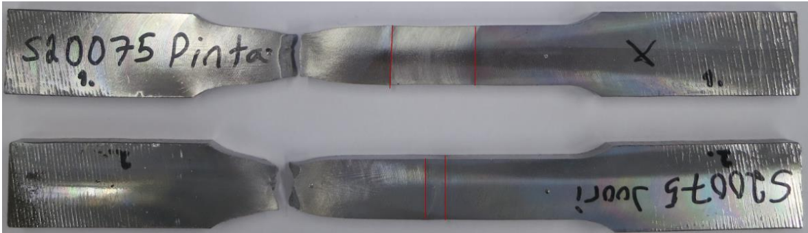
Figure 30. Test piece 4 S20075: transverse tensile test specimens
