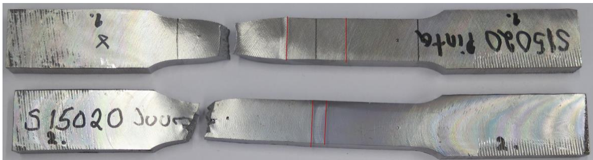
Figure 29. Test piece 2 S15020: transverse tensile test specimens
