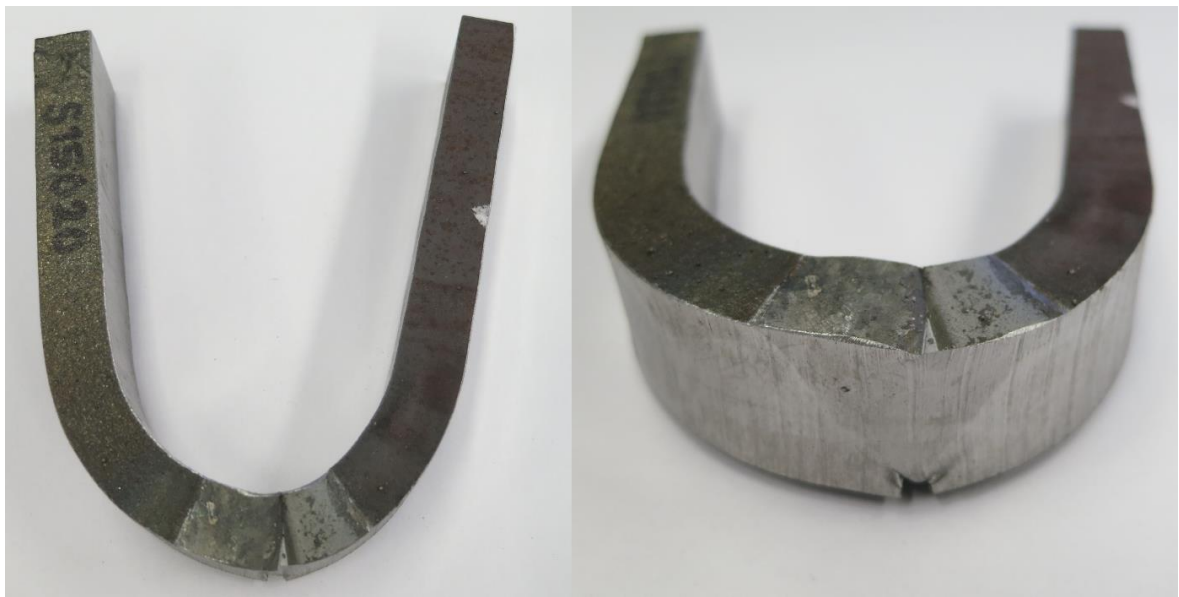
Figure 33. Test piece 2 S15020: bend test specimen
