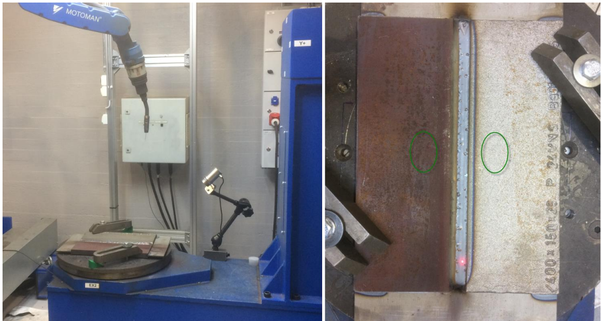
Figure 17. Welding setup and welded test piece
