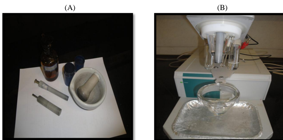
Figure 4.1: (A) Preparation of CPE (II, III) and (B) A conventional three-electrode system in Metrohm Computrace voltammetric analyser model 797VA.
