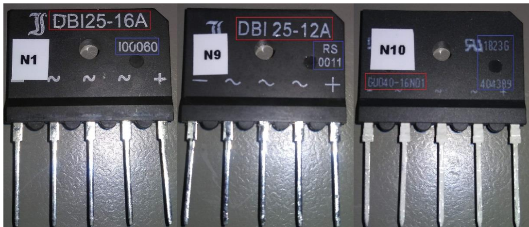
Figure 2.1. Three case types with different labeling layouts were recognized. Case type 1 is on the left, case type 2 in the middle and case type 3 on the right. Model names are marked with red and batch numbers with blue.
