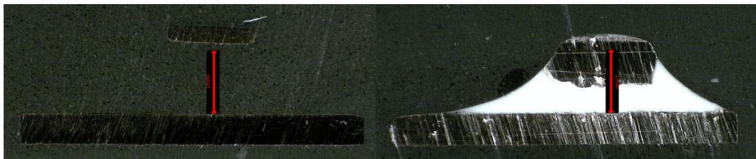
Figure 6.6. The insulation gap was significantly bigger on case type 3 compared to case type 1 and 2. Case type 3 also had the same epoxy as on the case between the live parts whereas case types 1 and 2 had a white dielectric between the live parts. On left case type 3 and on the right case type 2 insulation thickness between live parts.
