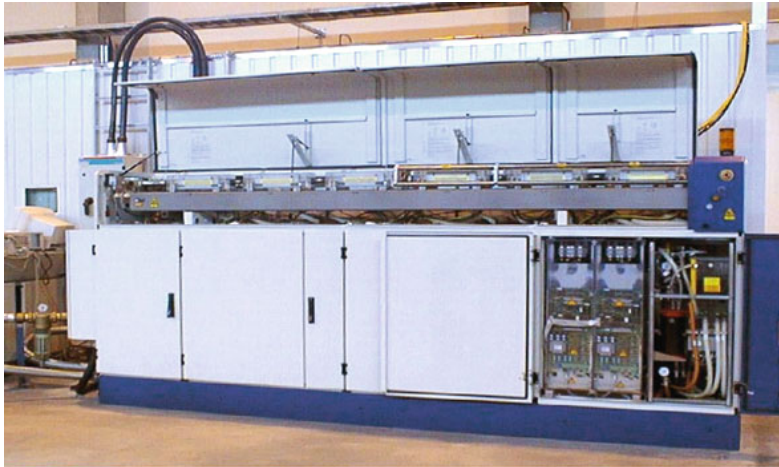
Fig. 6 3 kW Nd:YAG-laser used in the experiments
