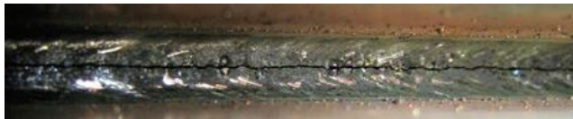
Fig. 11. Top view from above of narrow gap groove. A hot crack propagated to the surface of the laser arc-hybrid filling pass during the welding of multi-pass weld B22.
