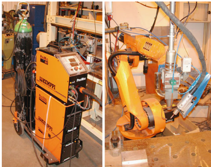
Fig. 7 Welding equipment used in the experiments. Left: Kemppi Pro MIG-welding machine, right: Hybrid welding head mounted in KUKA KR 15 robot
