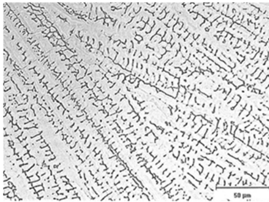
Figure 2.6: Weld microstructure which is a result from ferritic-austenitic- (Type F-A) solidification. Ferrite shows as dark skeletal like morphology. (Lippold and Kotecki, 2005)
