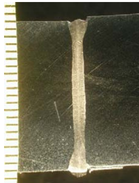
Figure 2.18: Example of a single-pass fibre laser weld produced on 20 mm thick butt-joint of AISI 316L austenitic stainless steel plates. Laser power 19 kW; welding speed 1.5 m/min; Focal position F = -4 (Kujanpää, 2014).
