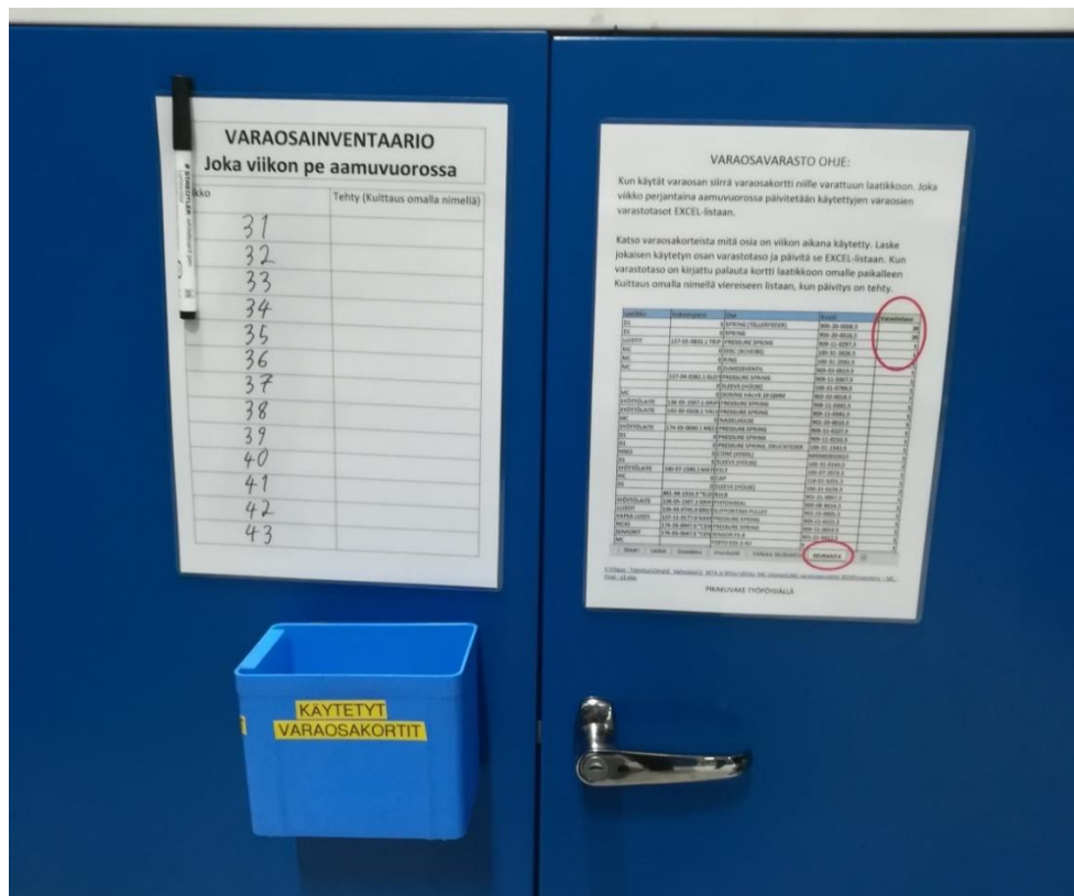
Figure 15. The instructions, signing sheet and a place for the used Kanban cards
