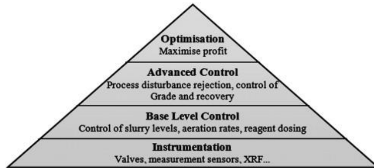
Figure 14. Process control system has four different layers, instrumentation, base level control, advanced control and optimization. Each of the layers communicate with the adjacent layers. (Laurila, H., et al., 2002)
