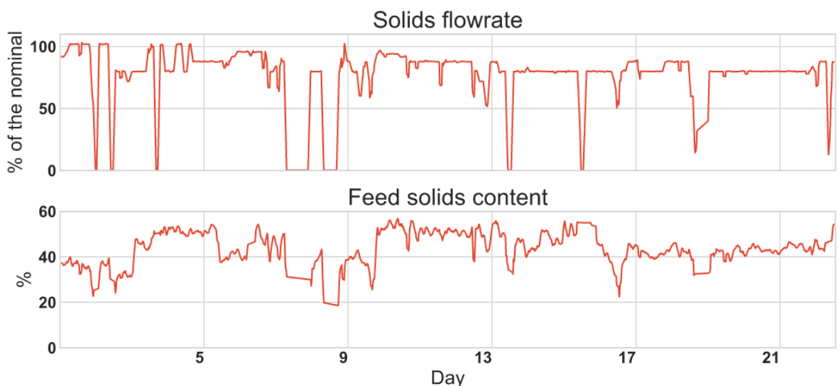
Figure 46. Feed's solids flowrate and solids content. The average for flowrate was 0.86 % of the nominal solids flowrate and 44.24 % for the solids content.
