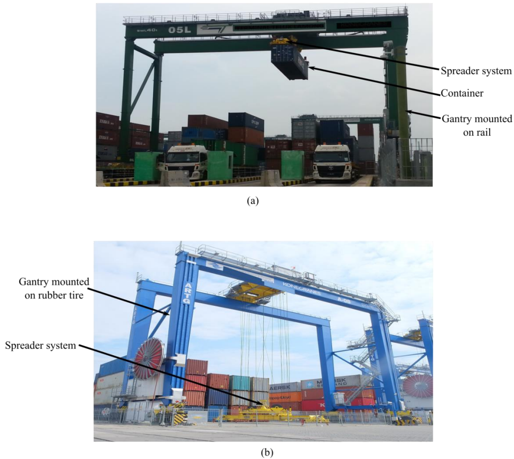
Figure 4 (a) An automated stacking crane (ASC) and (b) An automated rubber-tired gantry (A-RTG)
