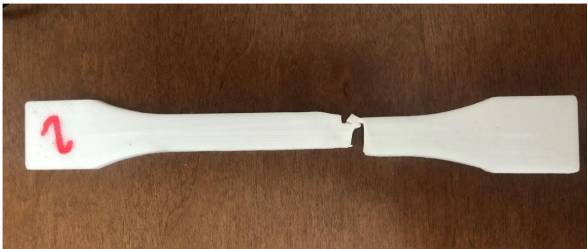
Figure 42. Test specimen B2 after tensile testing. The tear of the sample occurred slightly offset from the midpoint, but the tensile strength was still in line with other results.
