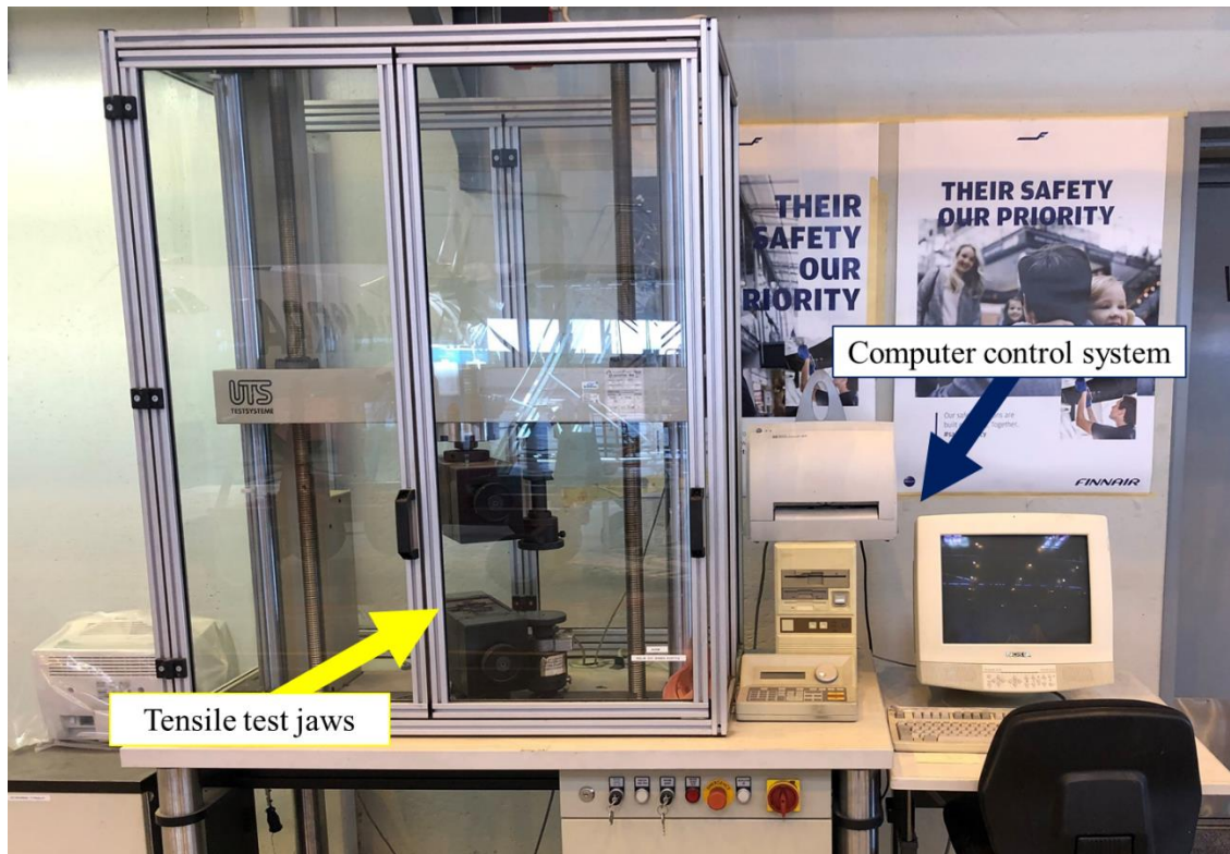
Figure 25. UTS system 100.20 tensile and compression testing machine setup.
