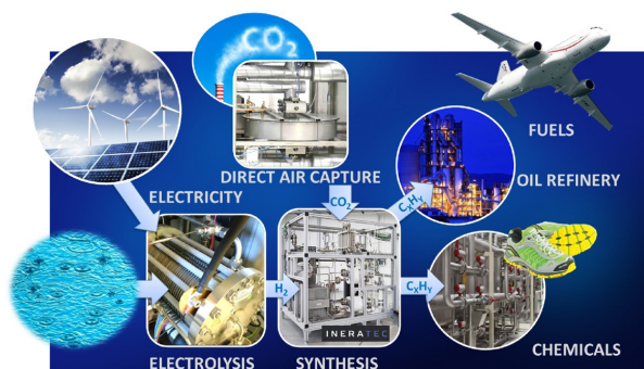
Fig. 1. The main idea of the SOLETAIR Power-to-X process producing CO 2 neutral hydrocarbons with renewable electricity.
