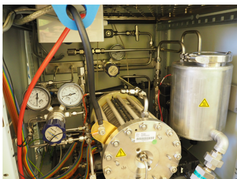
Fig. 1 – Water cooled E1050 differential pressure PEM water electrolyzer used in the experimental work.
