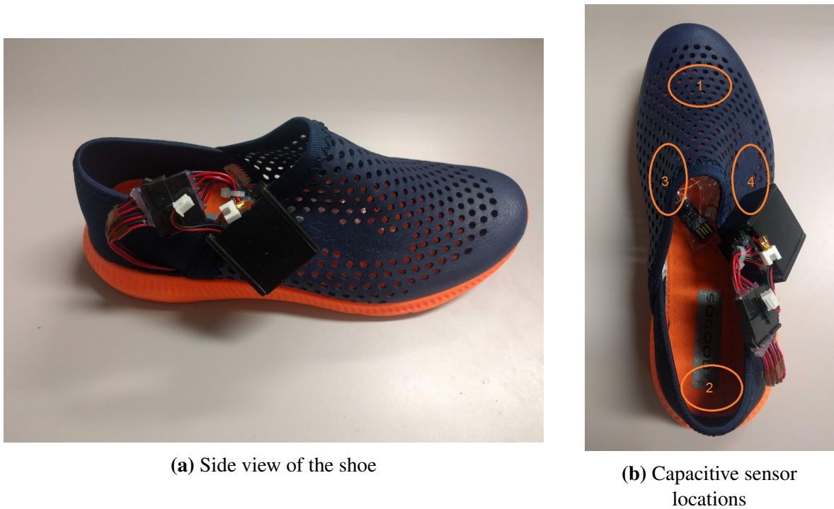
Figure 14: Capacitive sensor shoes to measure pressure used during experiments
