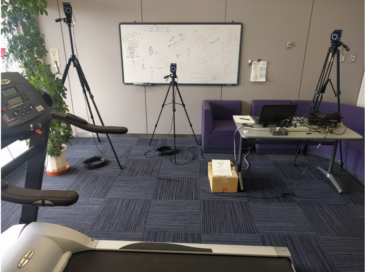
Figure 16: The complete set-up of the experiment: three motion capture cameras connected to the recording computer, aimed at the treadmill.
