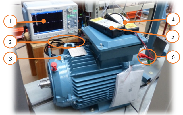
Fig. 9. Overview of the laboratory setup. 1: multi-channel oscilloscope Yokogawa DL850, 2: artificial neutral point connection, 3: the motor under test, 4: Rohde&Schwarz RT-ZD01 differential probe for shaft voltage measurement, 5: Rohde&Schwarz RT-ZD01 differential probe for the common-mode voltage measurement, and 6: brush connection to the shaft.
