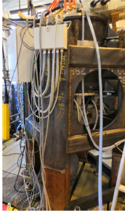
Figure 5.10. Hermetic steam turbo generator test rig. (From Publication V ).
