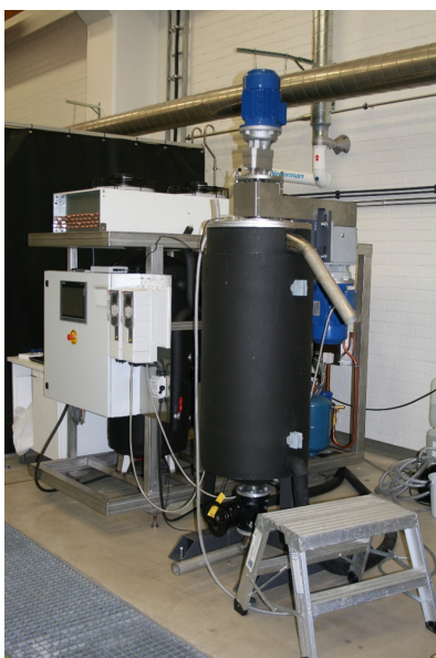
Fig. 3. Freeze crystallizer and cooling unit in the testing environment.
