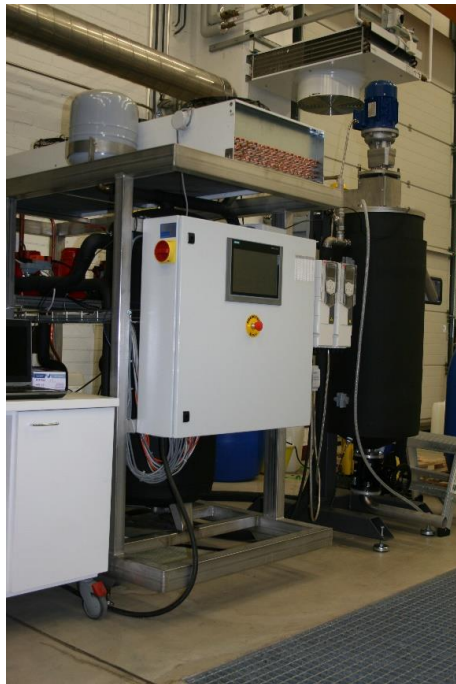
Figure 3.4: Experimental setup in the testing environment; the suspension freeze crystallizer and the cooling unit.
