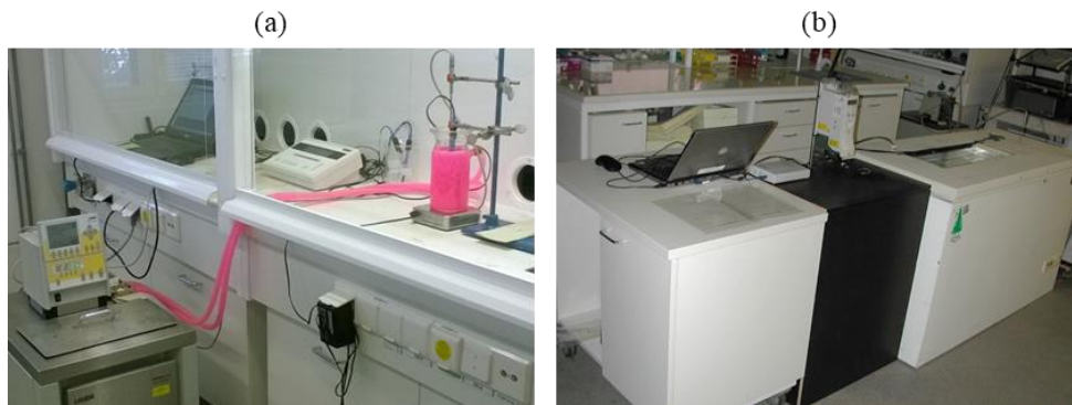
Figure 3.2: Experimental setups. (a) Freezing point depression determination. (b) Winter simulator.
