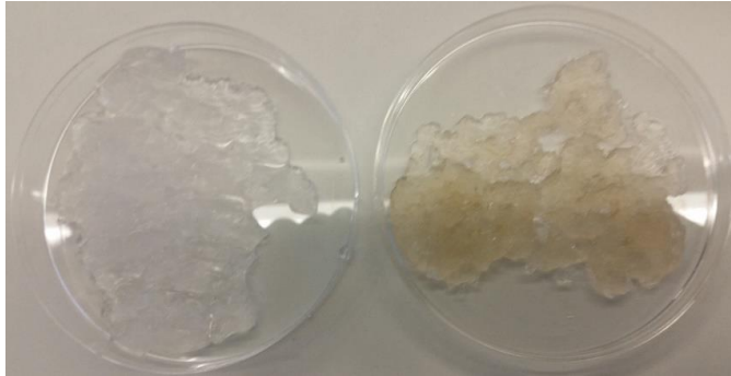
Figure 4.4: Colour differences in ice samples photographed after storing in a freezer. On the left is washed ice and on the right unwashed ice.
