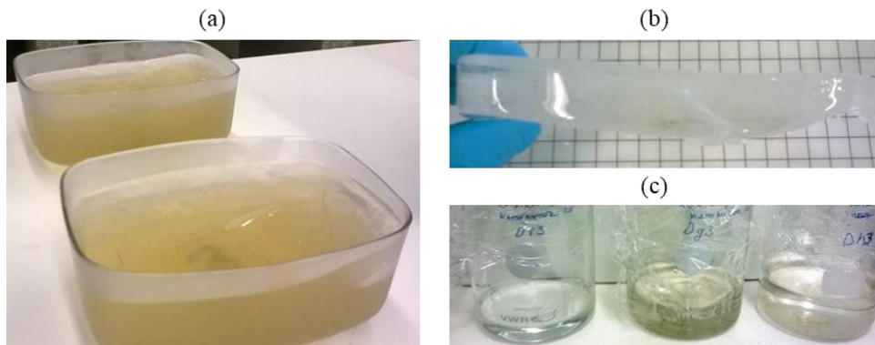
Figure 4.2: Municipal pre-treated wastewater after freezing. (a) Ice layers in crystallizer vessel. (b) Wedge-shaped ice piece. (c) Melted ice samples.
