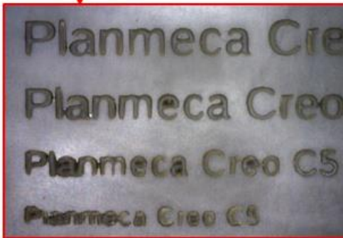
Figure 49. Experiments and enlarged figures of the experiments 2.2.4 and 2.2.5, second test round where only exposure time was varied.
