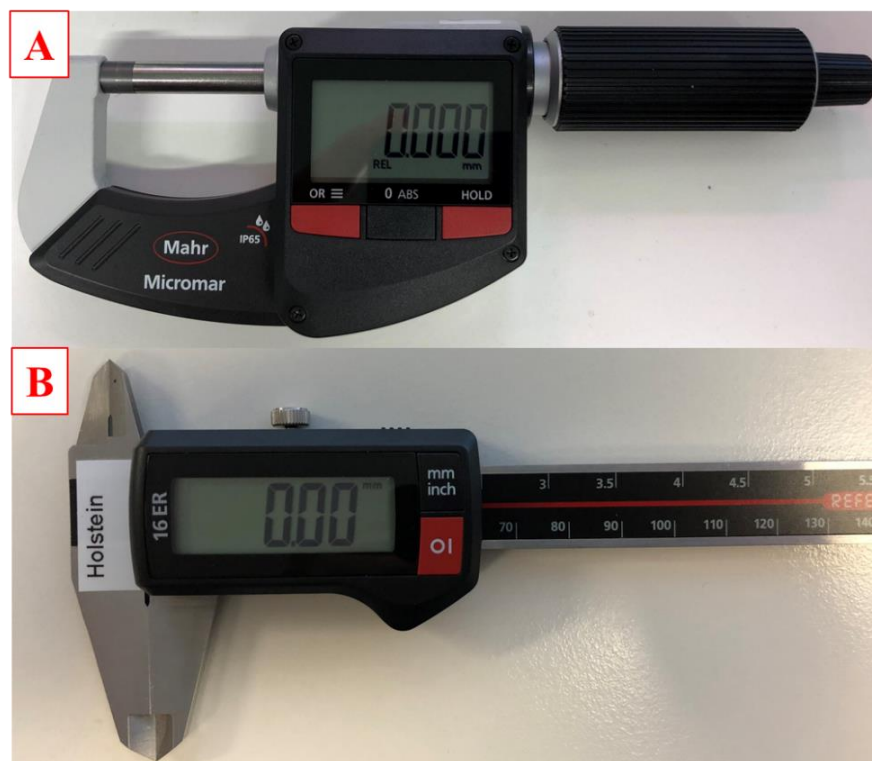
Figure 33. Measurement tools, above (A) digital micrometer Micromar 40 EWR(i) from Mahr and below (B) slide gauge MarCal 16 ER from Mahr.
