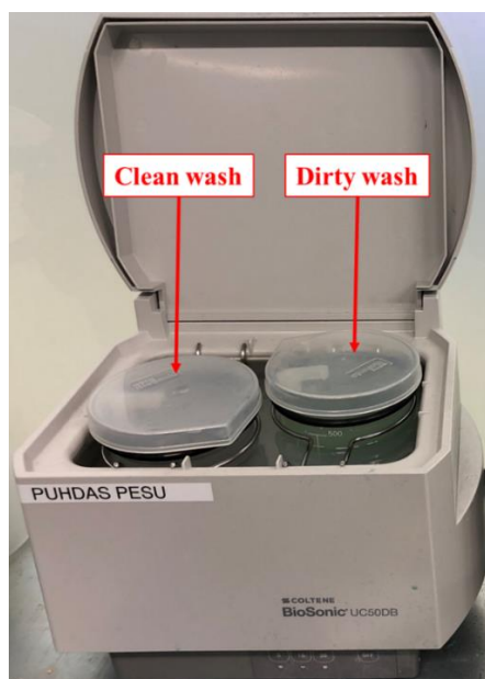
Figure 32. BioSonic UC50DB ultrasound washer filled with water and classes, for dirty and clean wash, filled with Emplura Propanol-2.
