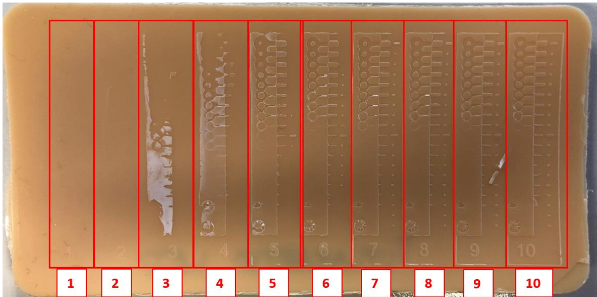
Figure 27. Anycubic Photon quick exposure time finder print printed at Planmeca with Creo C5.
