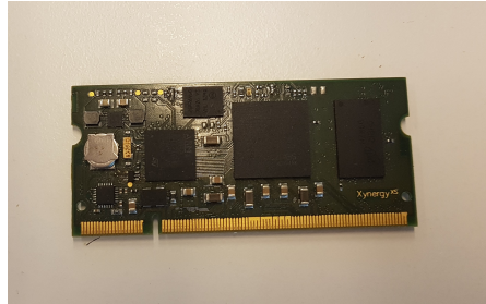
Figure 1.6. XynergyXS board used to control the AC/DC power supply.
