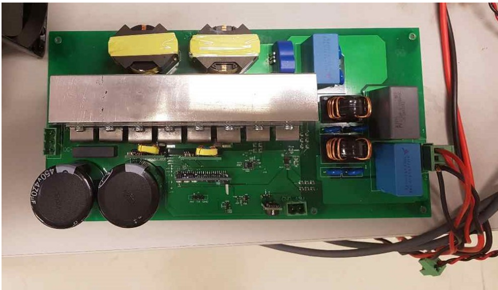
Figure 3.4. Single-phase inverter with the EMI filter and the FPGA control used for the experimental measurements.
