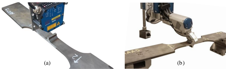
Figure 3.6: (a) geometry measurement using a 2D coordinate measuring device, and (b) XRD residual stress measurement device.
