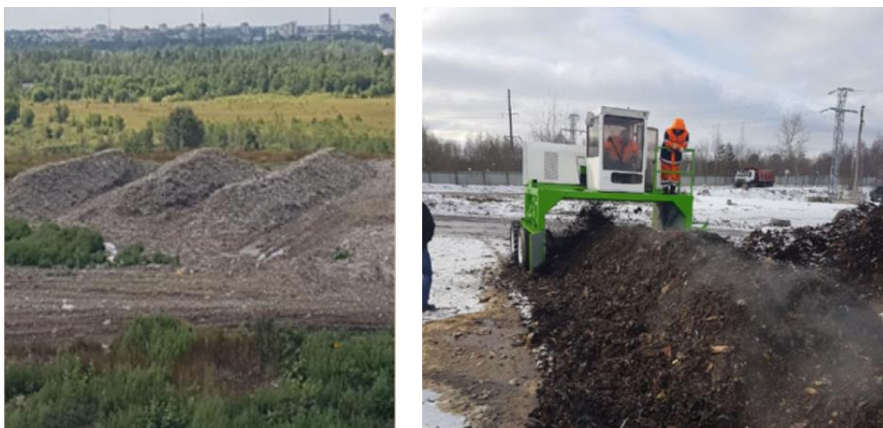
Figure 5. Windrow composting of MSW undersize fraction, Novyy Svet landfill (Malyukhin et al., 2018)
