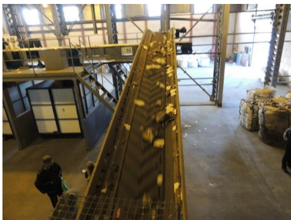
Figure 6. Paper fraction, which was sorted out by an optical separator, Starobryadcheskaya waste processing plant (RazDelniy Sbor, 2020c)
