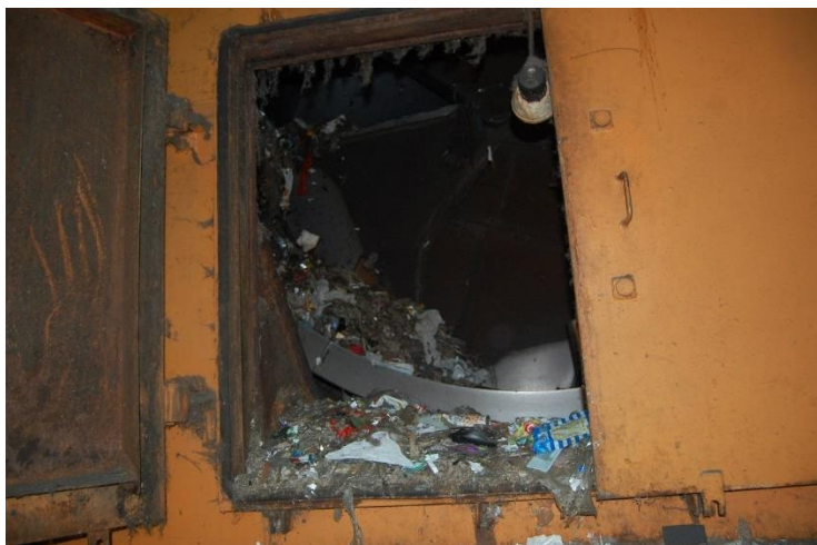
Figure 3. Screening reject that is composted in rotary drums at MPBO-2 (RazDelniy Sbor, 2015)
