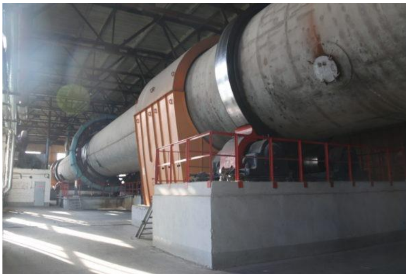
Figure 2. The drum for composting of organic waste at MPBO-2 (MPBO-2, 2018a)
