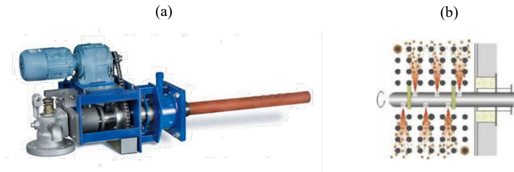
Figure 15. (a) Rotating soot blower (Clyde Bergemann 2020b). (b) Basic operation principle of a rotating steam soot blower (Clyde Bergemann 2020b).
