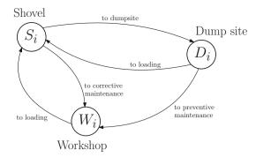
**Fig. 5** Scheme of the agent's movements on a map inside the maintenance module between its sub-systems.  $S_i$  represents a generic shovel site,  $D_i$  represents a dump site, and  $W_i$  a workshop
