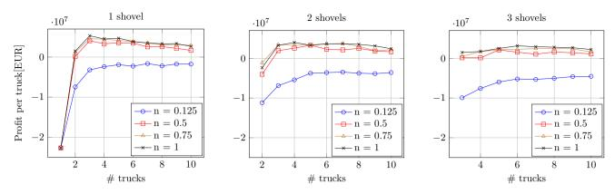
Fig. 14 The profit per truck is plotted as function of the number of trucks for different maintenance policies
