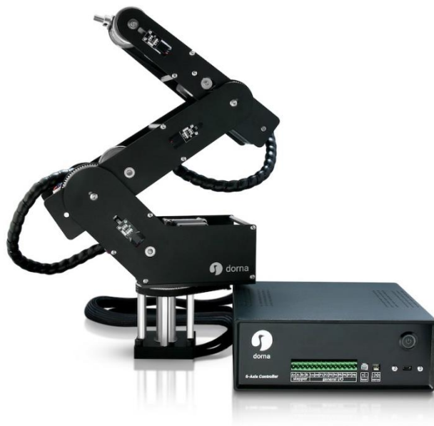
Figure 4. DORNA 2 robotic arm and control unit (DORNA Robotics, 2020)
