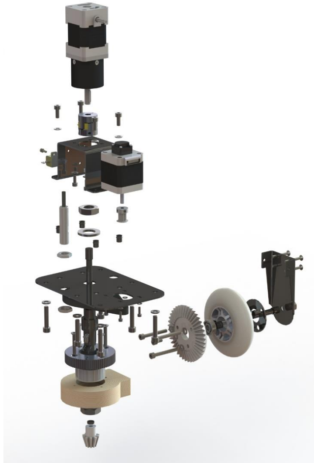
Figure 10. Exploded wheel module assembly
