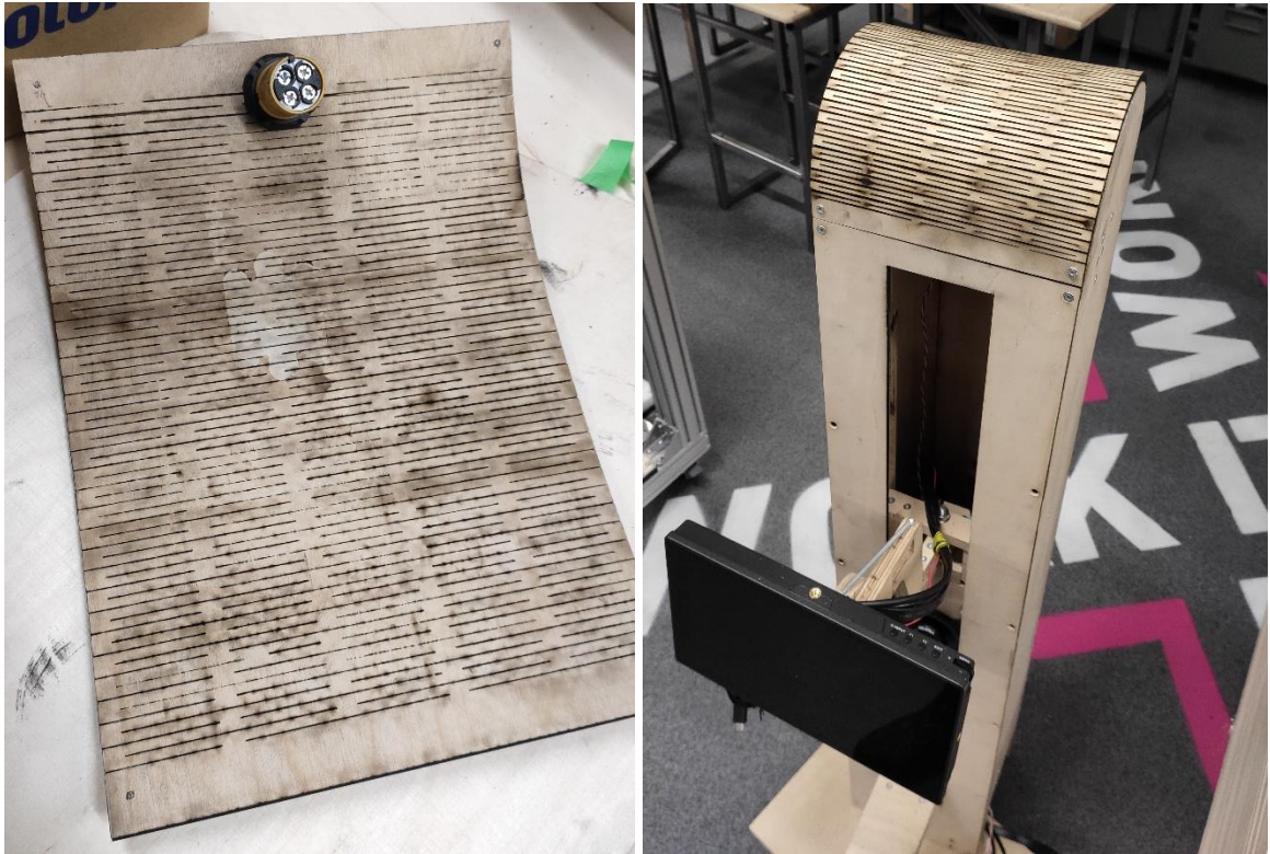
Figure 23. Tower top a) Laser cut to include flexibility as thermoformable plywood is not available b) In the tower assembly
