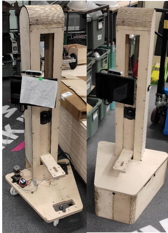
Figure 28. Robot frame propped up a) with wheels and no side plates b) with side plates, top plate and no wheels
