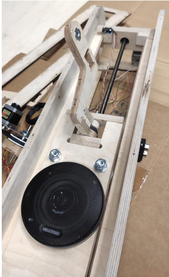
Figure 22. Linear plate assembly inside the tower assembly
