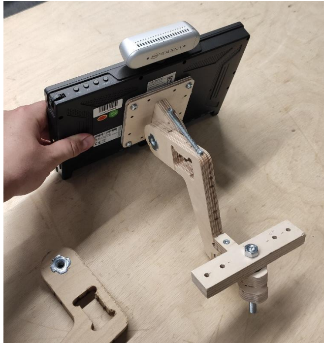
Figure 17. Beginning screen arm mechanical assembly
