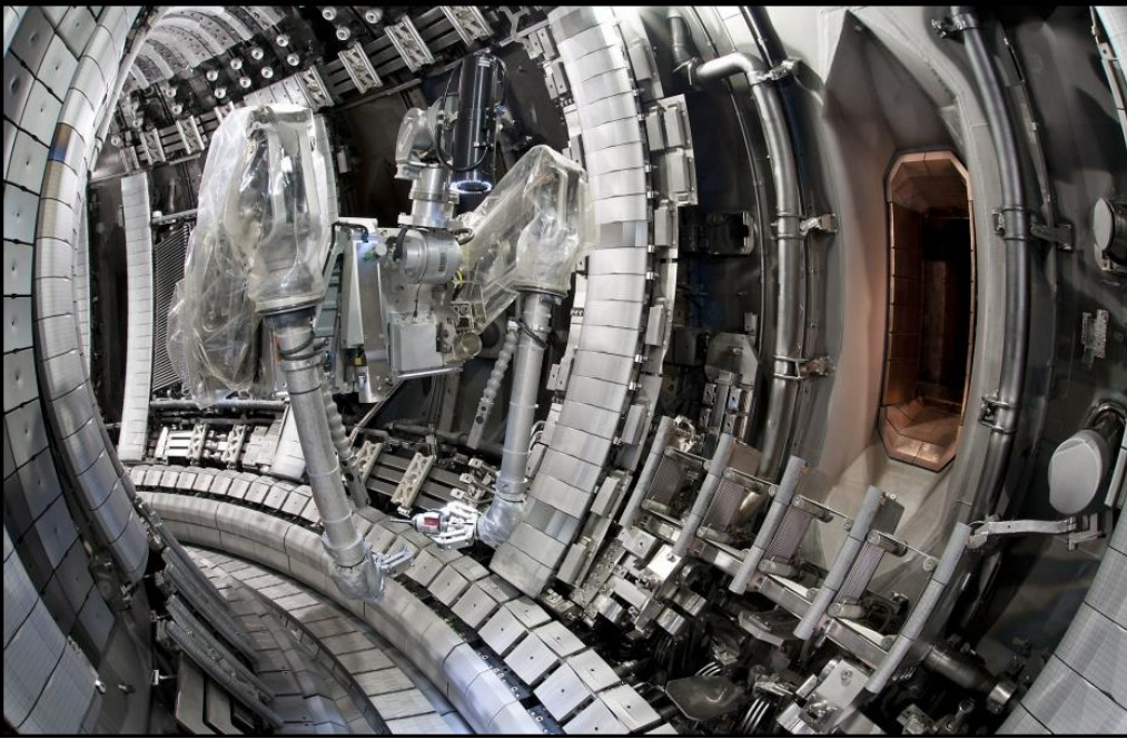
Figure 1.3: JET device end dual arm system Mascot (Wikipedia, 2021)
