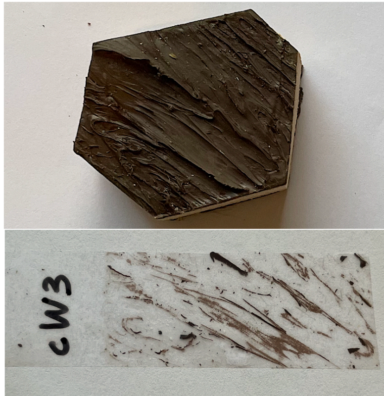
Figure 17. The destruction nature of coating #3
