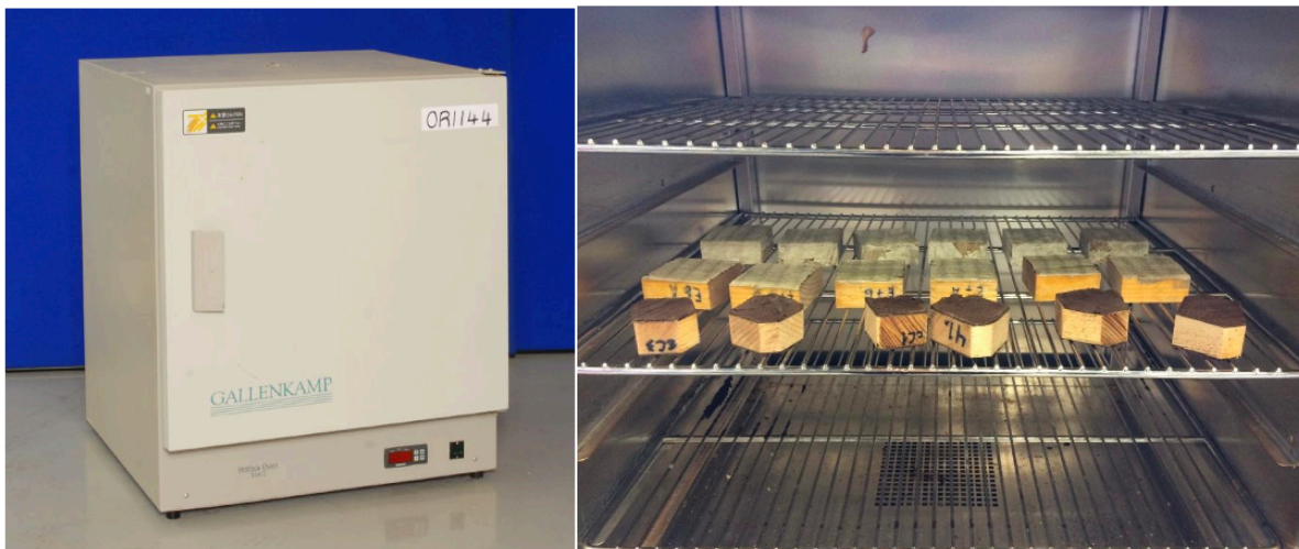
Figure 11. The position of coated samples into the drying cabinet.
