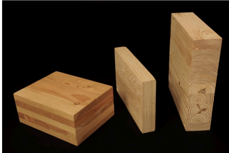
Figure 2. Mass timber. CLT, LVL, and glulam presented from the left to the right sides (Jakes et al. 2016).
