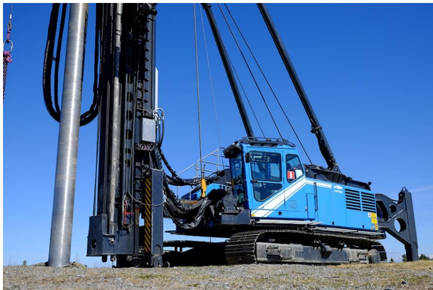
Figure 5. MPx90 multipurpose drilling rig (Junttan 2020b).
