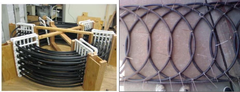
Figure 40. Different Spiral Helical coil geometries. (Hansen, 2011)
