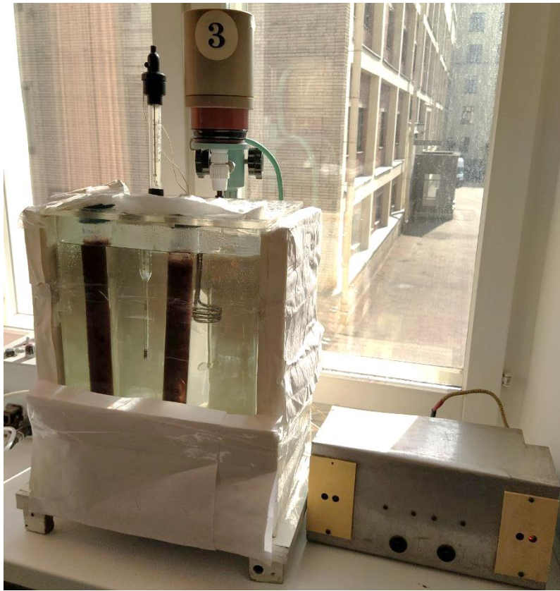
Figure 24. Temperature control unit with two filled measuring cylinders
