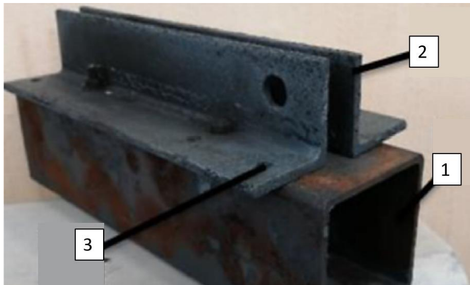
Figure 6. Clamping device used for rigid fixing. (Voropaev et al. 2020, p. 2).
