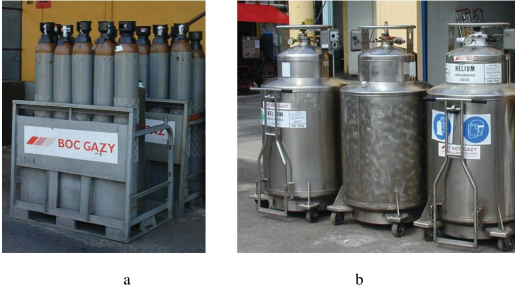
Figure 3.16: Small-volume helium storage containers. (a) Cylinders of gaseous helium. (b) Dewars of liquid helium (National Research Council, 2010).
