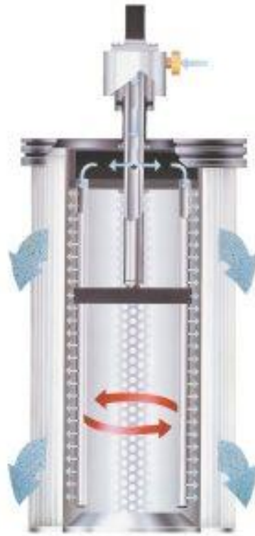
Figure 5.7: Rotating pressurized air cleaning nozzle.
