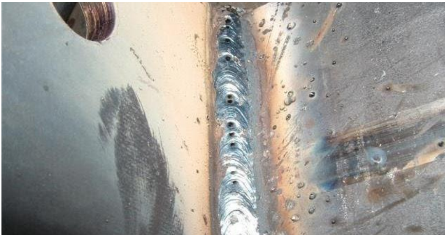
Figure 4.7: Porosity defect after welding.
