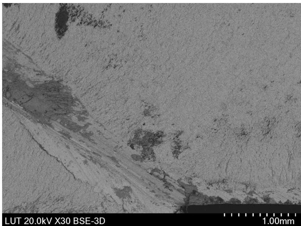
Figure 21. SEM picture of the crack growth at the ridge.
