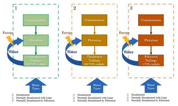
Fig. 1. Simplified scheme of every option of tailings management and water treatment considered in the study.
