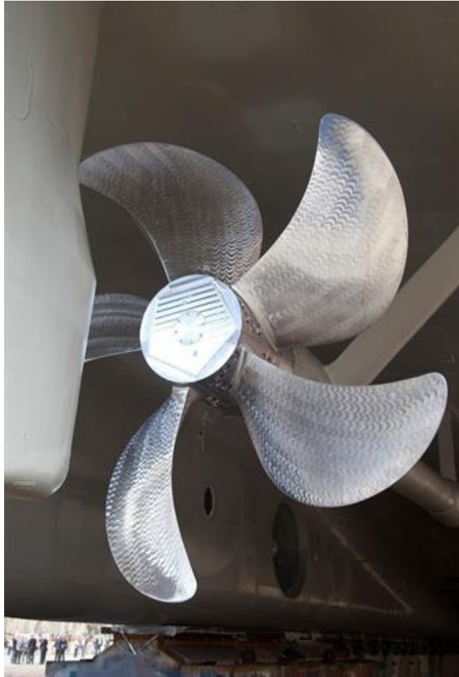
Figure 6. Built-up fixed pitch propeller (Wärtsilä, n.d. a)
