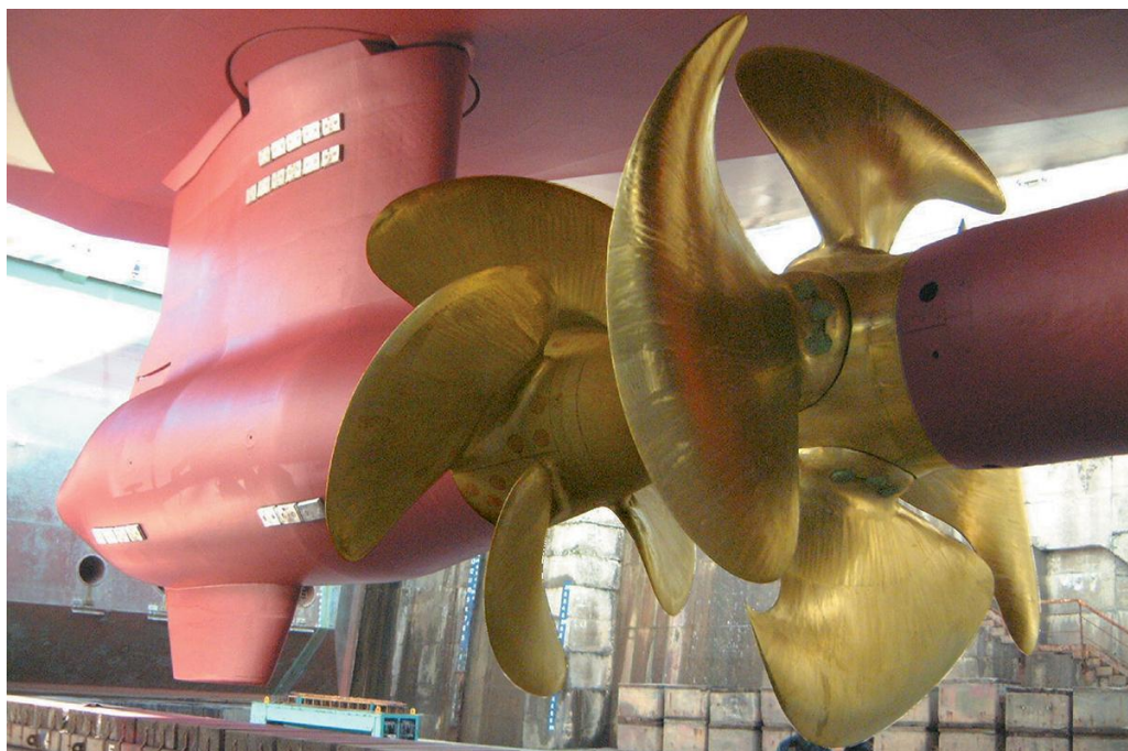
Figure 10. Contra-rotating propeller variant with podded propeller (ABB, 2004)
