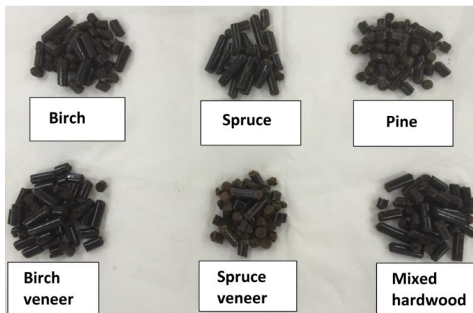
Figure 12: Visual differences of torrefied pellets. Birch pellets had the highest mechanical durability (97.4 w-%) and pine pellets had the lowest (91.8 w-%) (Publication II).
