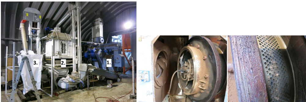
Figures 8 and 9: On the left is 1. the pelletizing unit, 2. screening unit, and 3. bagging unit (Publication II). On the right is a closer look at the iron matrix (Publication II).
