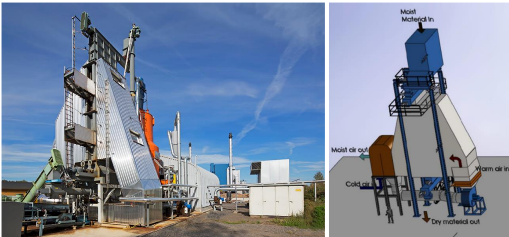
Figures 5 and 6: On the left is the pilot plant of Torrec Ltd in Mikkeli, eastern Finland (Publication I). On the right is a single-phase process in which both drying and torrefaction occurs (Publication I).
