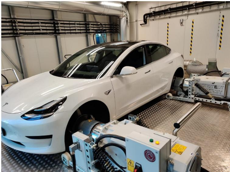
Figure 5: Photo of the testing laboratory. Tesla mounted on a four-wheel drive dynamometer.
