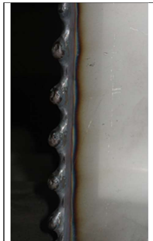
Fig. 6. Example showing weld sagging tendency occurring in vertical welding position.
