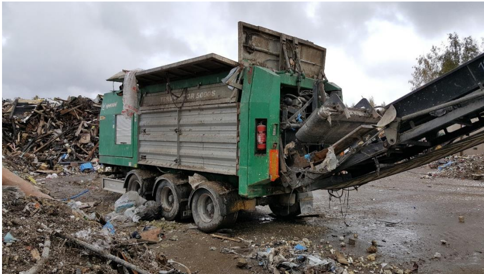
Figure 3. Mobile Terminator 5000S crusher crushing mixed C&D waste © Havukainen
