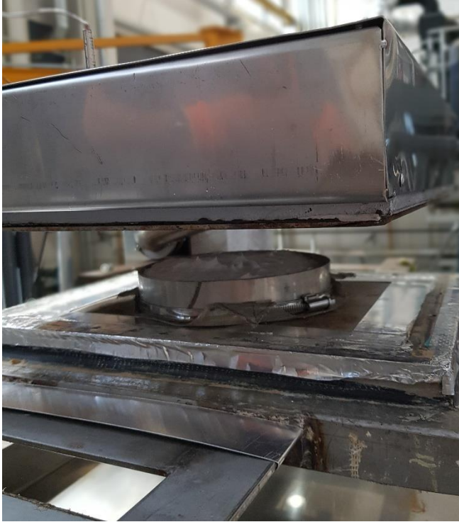
Figure 22: Sample getting dried under the air impingement box.
