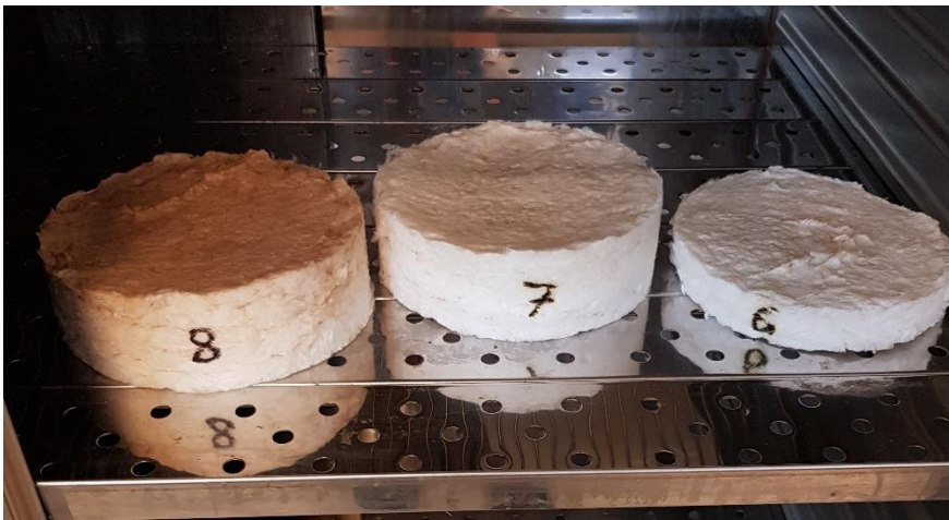
Figure 31: Impingement air temperature effect to the surface of the samples. 150 °C (samples 6 and 7) and 200 °C (sample 8) air temperatures.
