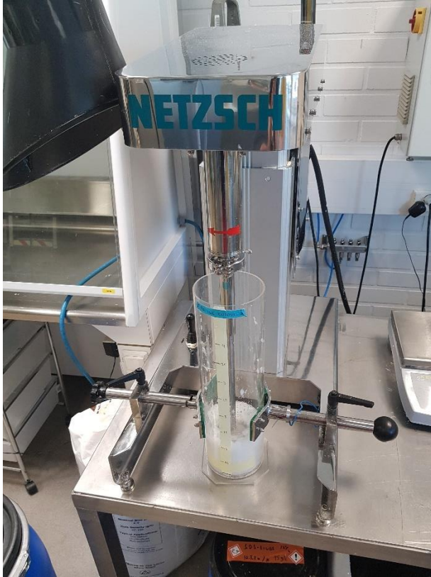
Figure 13: Netzsch mixer that was used in foam generation.
