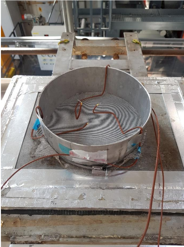
Figure 20: Thermocouple wires connected to sample mold.
