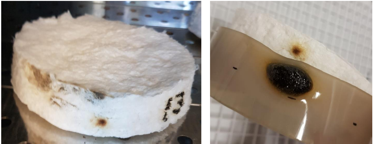
Figure 43: The effect of the burn damage to the sample and sample mold.
