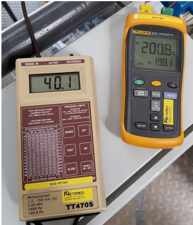
Figure 16: Mikor TT4705 pressure meter (left) for jet velocity monitoring and Fluke 54 II thermometer (right) for jet temperature monitoring.
