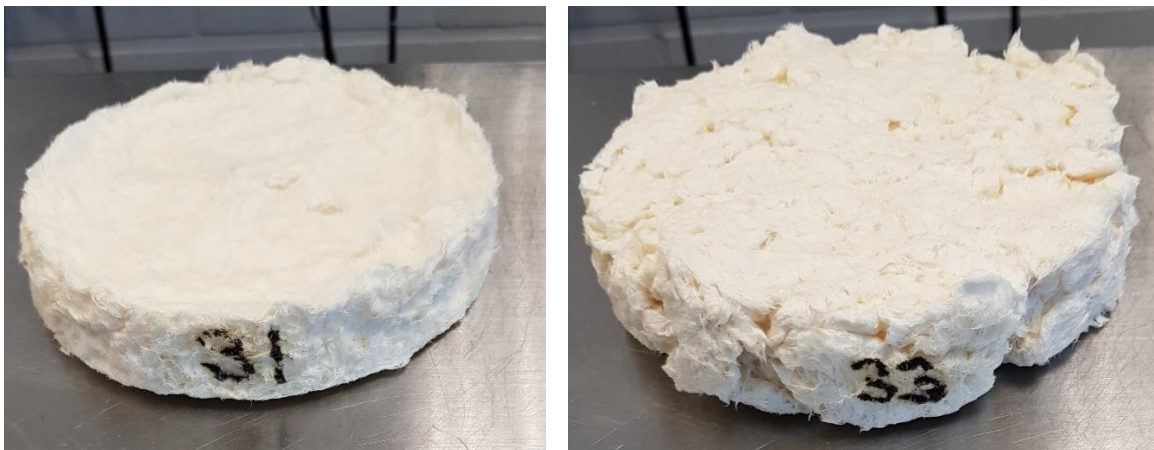
Figure 47: 5 % (left) and 10 % (right) consistency CTMP samples dried with 100 % microwave power and 39 mm mold.
