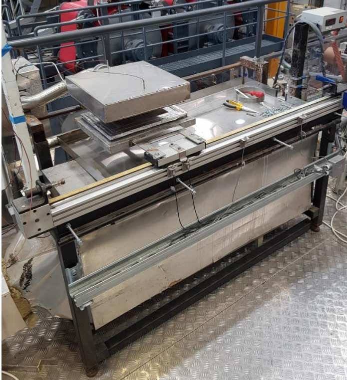
Figure 15: Air impingement box mounted to supportive table.
