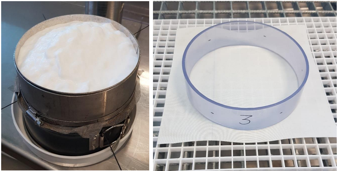
Figure 14: Examples of drainage and drying setup for impingement (left) and microwave (right) drying.
