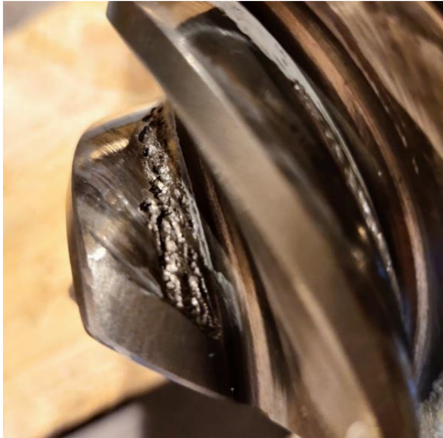
Figure 11. Detail from Figure 6 showing pitting damage on gear flank near root and scuffing near tip diameter
