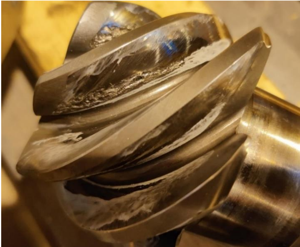
Figure 10. Scuffing and pitting damage in gear flanks
