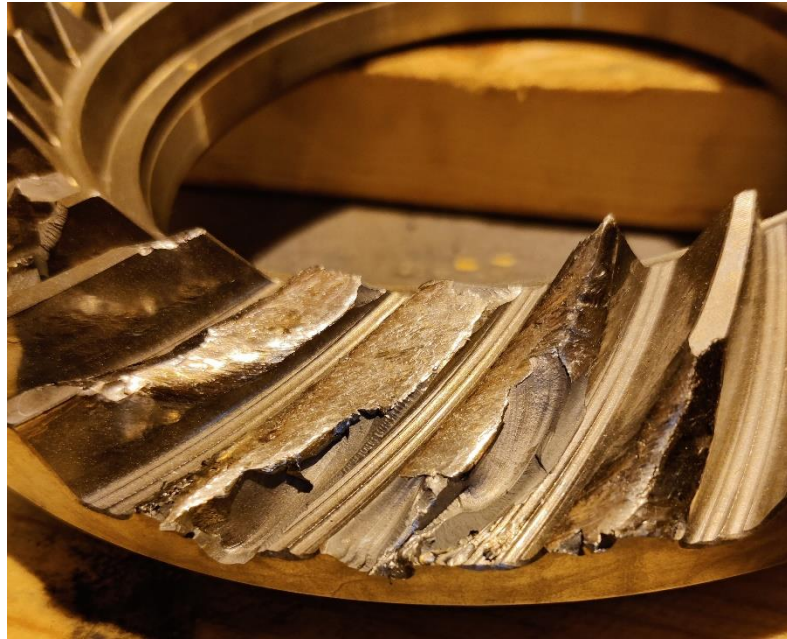
Figure 12. Gearwheel with damaged teeth
