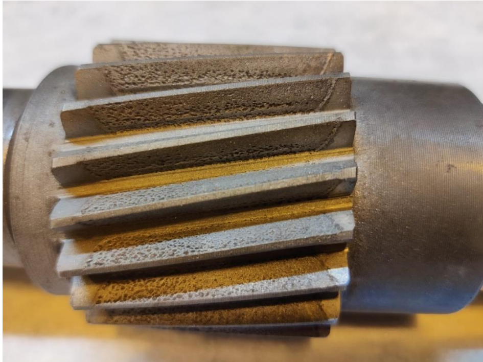
Figure 8. Pitting in gear flanks
