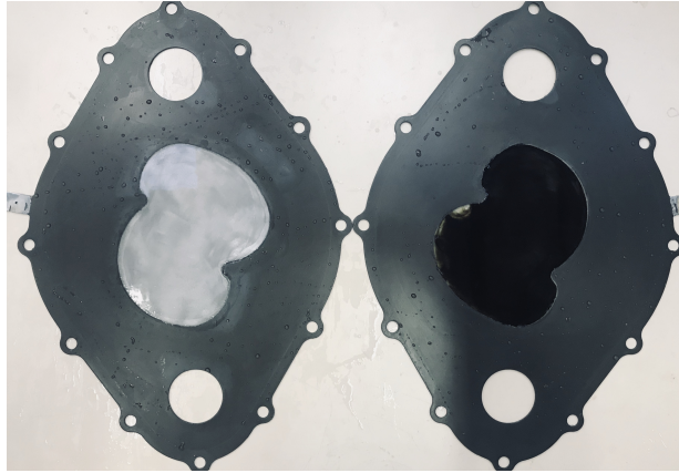
Figure 4.9: Images of the third electrolyzer prototype before and after deposition of Co-Pi, published in Publication V .
