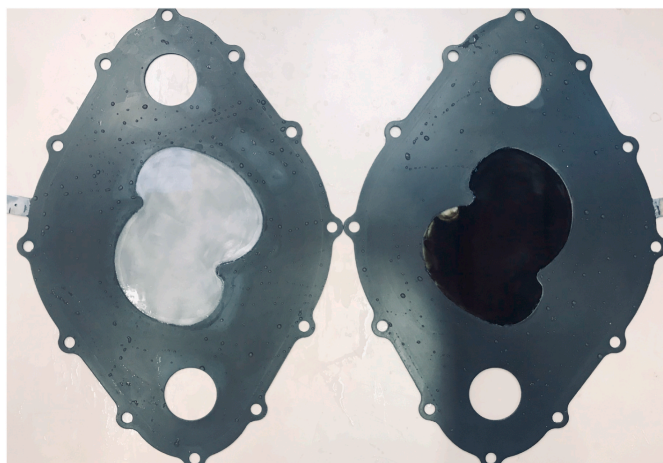
Fig. 5. Photo of the electrolyzer stack plates before and after coating with the CoPi catalyst.
