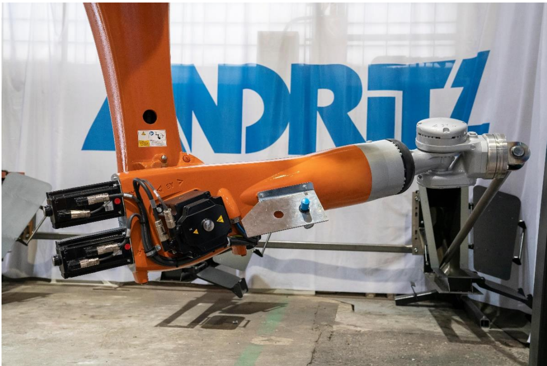
Figure 1. The Smelt Spout Robot at the testing environment in ANDRITZ Warkaus Works in Varkaus, Finland (Andritz 2019).
