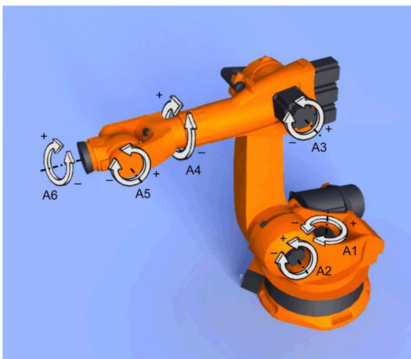
Figure 8. Joints of the 6 DOF industrial robot (KUKA 2021e, p. 85).
