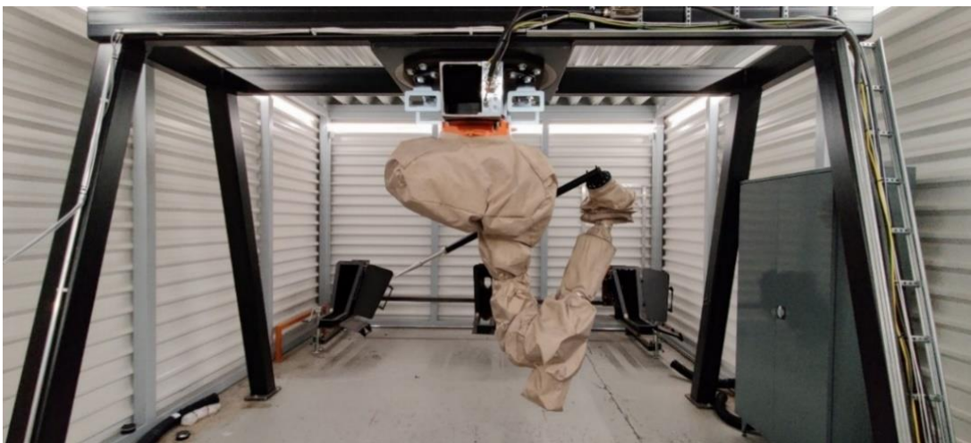
Figure 31. Practical tests were performed in the test environment that included a steel support structure, three smelt spouts, and the robot.
