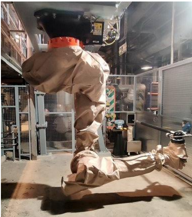
Figure 24. A tool cleaning machine removes the solidified melt on the surface of the tool.
