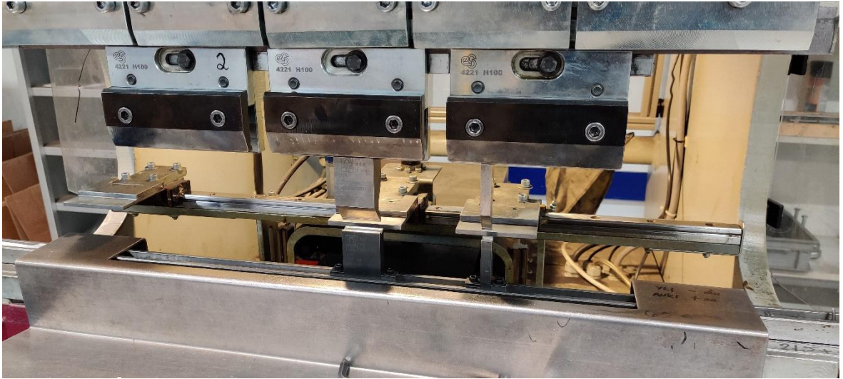
Figure 2. Multi-tool setup on press brake.
