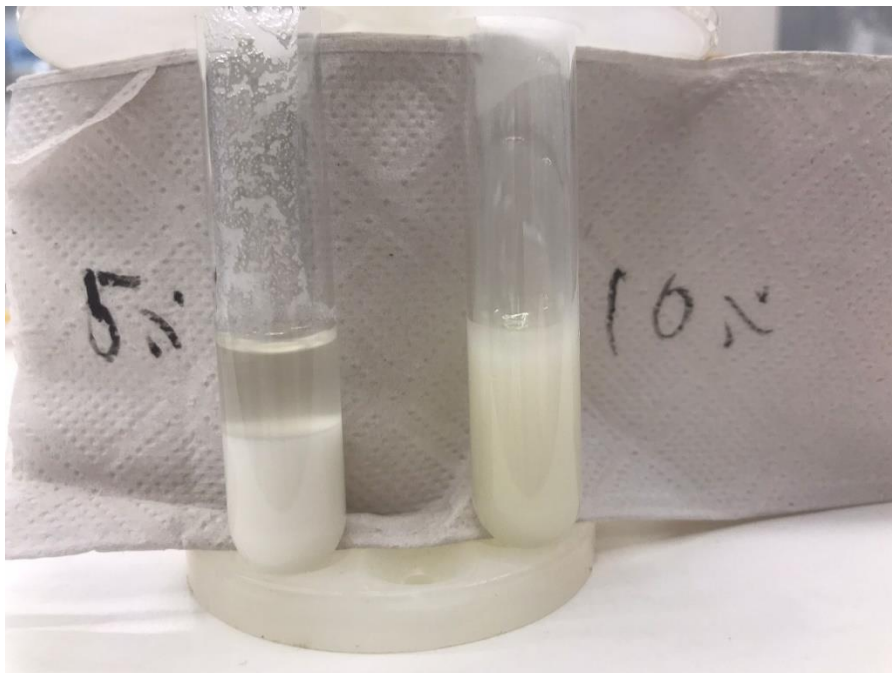
Figure 30 Microcrystalline cellulose in 5w% and in 10w% NaOH concentration with L/S 9
