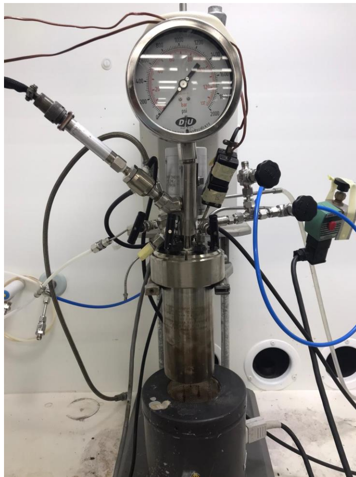
Figure 16 Autoclave used in the experiments
