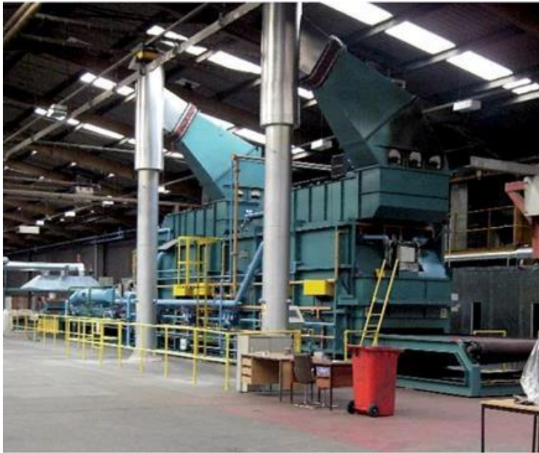
Figure 8. Industrial-scale pyrolysis process operational in ELG Carbon fibre, UK [43]
