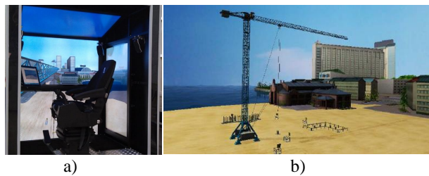
Figure 4. (a) Cabin of the multibody dynamics simulator and (b) model of a Liebherr 112EC-B8 tower crane.
