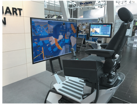
Figure 13. Simulator has an authentic operator chair with controls and touch screen user interface.
