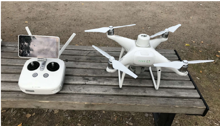
Figure 5. Phantom 4 RTK drone and controller.
