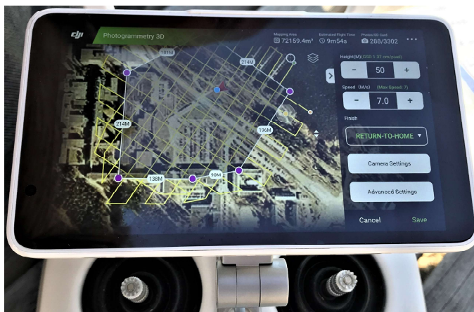
Figure 6. Flight maps of the chosen area for photogrammetry.
