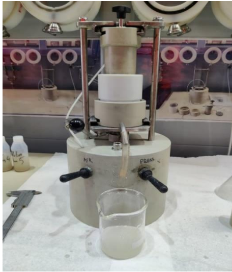
Figure 35 Metso Outotec Larox® Labox 25 (Metso Outotec)
