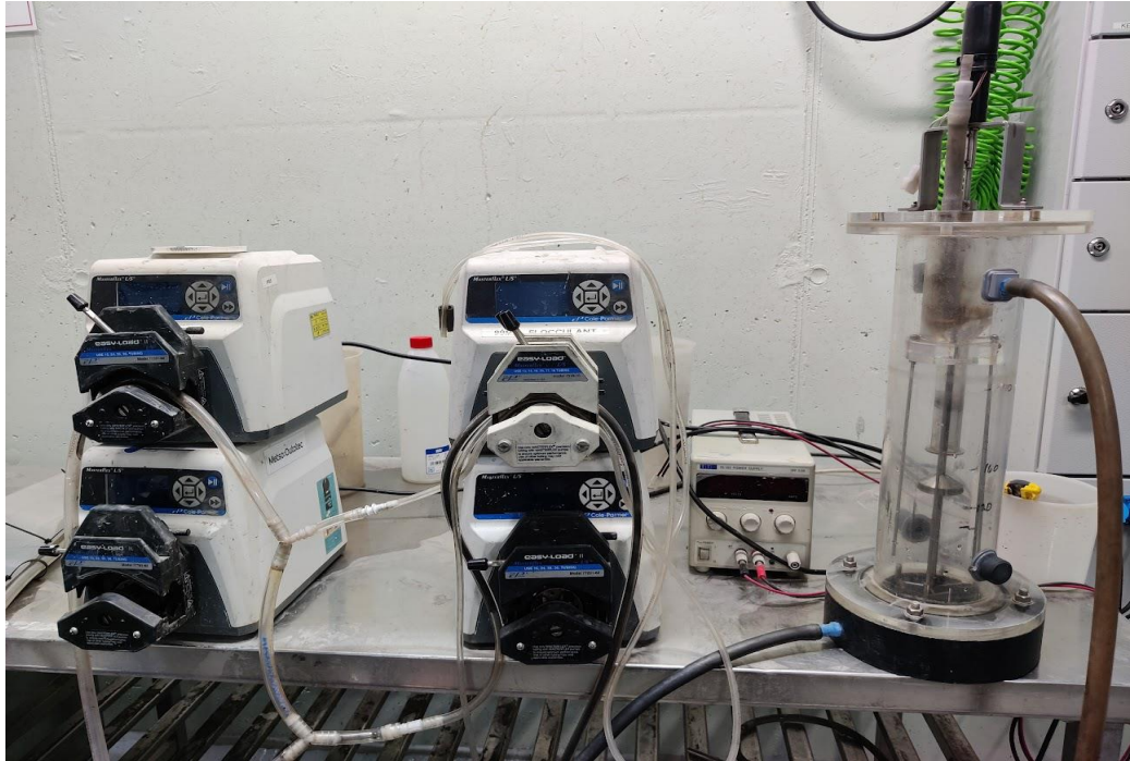
Figure 16 99mm diameter high-rate thickener (Metso Outotec)
