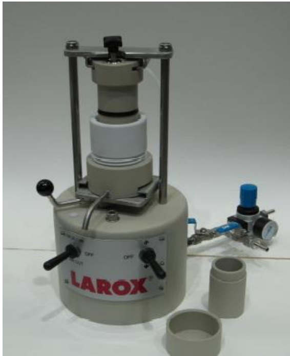
Figure 17 Metso Outotec Larox® Labox 25 bench scale unit (Metso Outotec)
