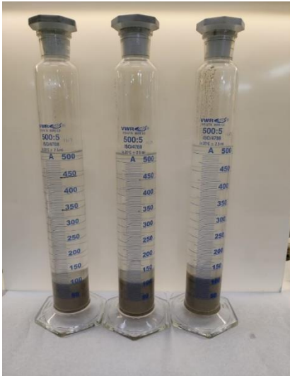
Figure 29 Flocculant screening tests for Composite tailings. From left to right; M10, M155 and M5250 respectively
