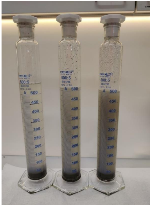
Figure 20 Flocculant screening tests for graphite tailings at pH 6. From left to right; M10, M155 and M5250 respectively
