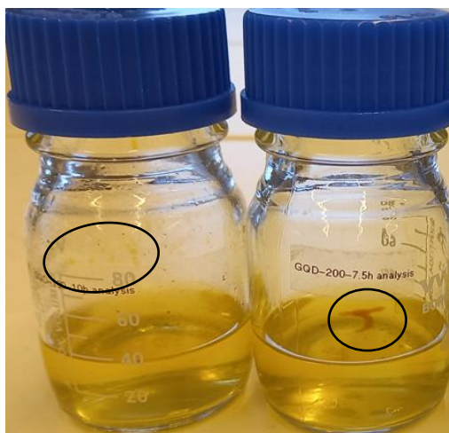
Figure 22. Synthesis results with brown aggregation starting from left to right Sam1- GQD-190-10h, and Sam1- GQD-200-7.5h
