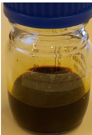
Figure 31. The hydrothermal treatment product using D(+)-Glucose anhydrous as the precursor
