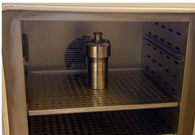
Figure 10. Filled Teflon autoclave placed inside the Termaks 8000 oven
