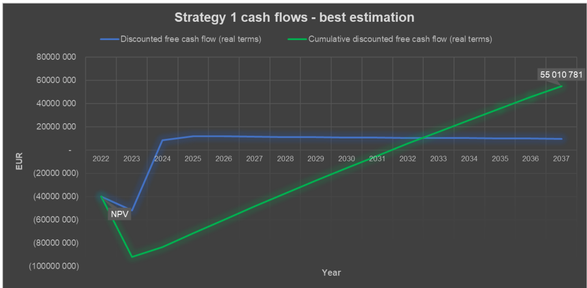
Figure 9. Discounted free cash flow and cumulative discounted free cash flow (real terms) of strategy 1 (build in one phase) best estimation scenario.
