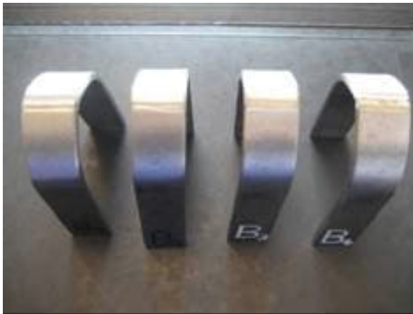
Figure 5.12: Bend test specimen welded with laser-hybrid welding.
