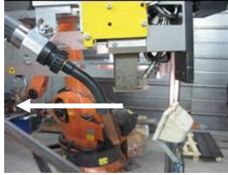
Figure 2. The GMA welding torch and laser optics. The arrow shows the welding direction.
