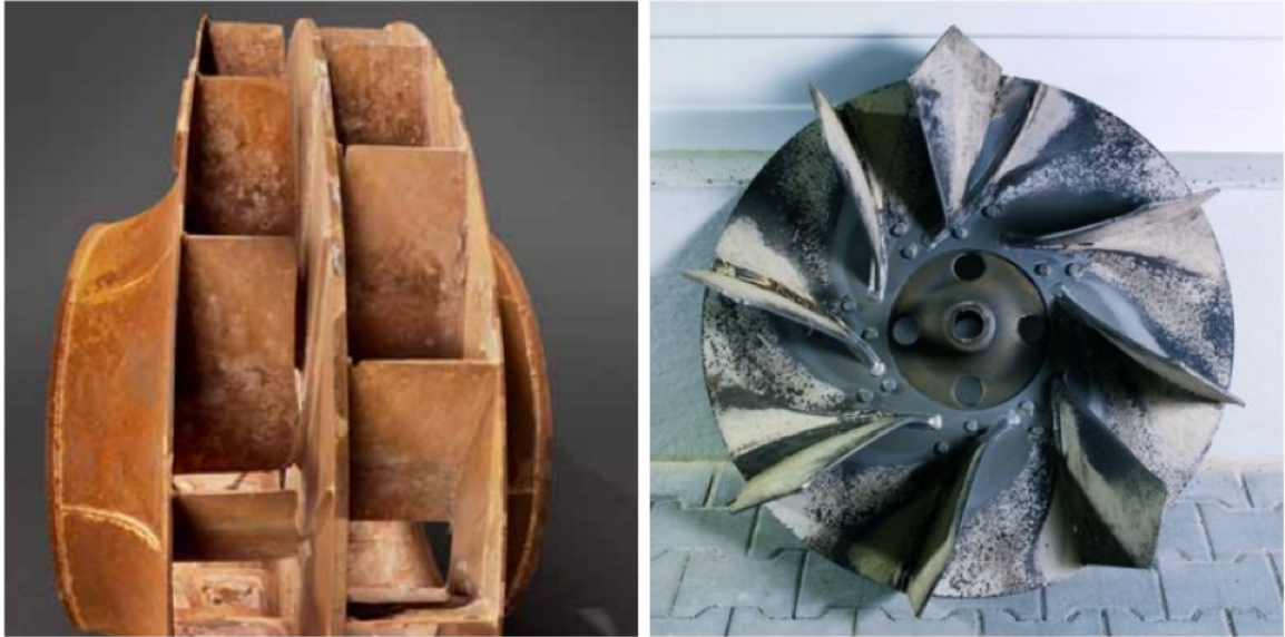
Figure 12. From the left: a worn-down impeller without protective coating and a fan impeller, used in the timber industry, with critical wear and some broken and cracked blades (Venti Oelde 2023b, 2 and Venti Oelde 2023a).
