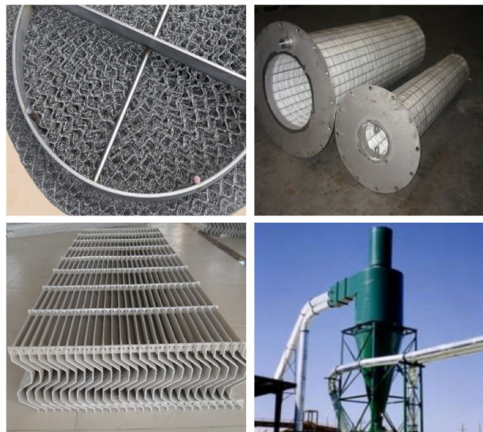
Figure 33. Droplet separator technologies. Left to right, on the upper row are pictures of a wire mesh separator (Alino 2022) and a cylindrical fibre separator (Ningbo T.C.I Company 2022a). General depictions of vane (Ningbo T.C.I Company 2022b) and cyclone separators (Ganga Reddy and Kuppuraj 2015) are seen on the lower row.
