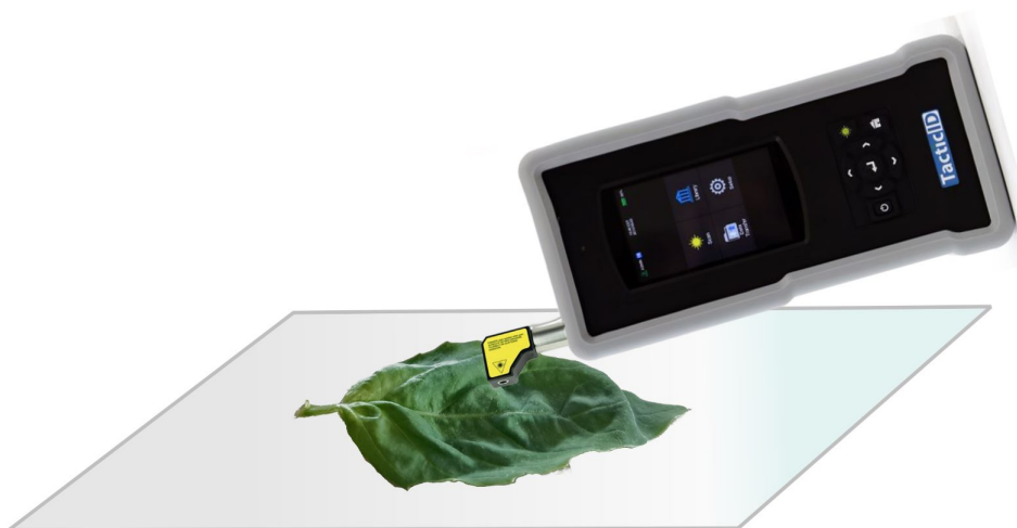
Figure 7. Schematic of a measurement setup, instrument fitted with the right angle adapter.
